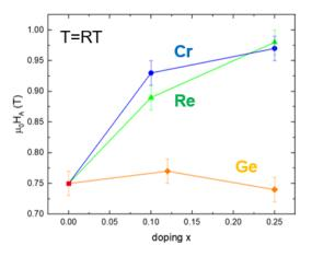
Anisotropy field as a function of Re, Cr and Ge content
