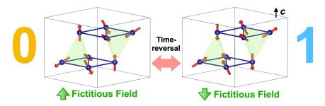
Two possible antiferromagnetic domains realized in CoTa3S6, which are converted into each other by time-reversal operation and characterized by the opposite sign of ficitious magnetic field.
